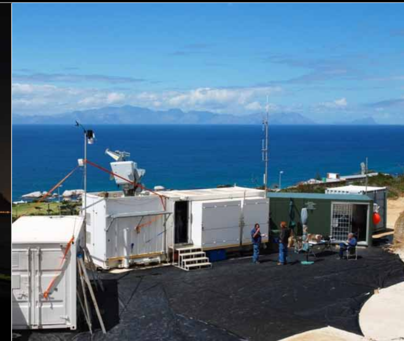
MecORT deployed above Simons Town during October 2010 for the first AwareNet integrated sensor experiments. Data from the MecORT and Spider radars, electro-optical and signal intelligence sensors, IFF transponders as well as AIS and GPS position reporting systems were collected via a real time sensor network, integrated into a sensor fusion database, geo-referenced and displayed on a GIS-based common operating picture.
