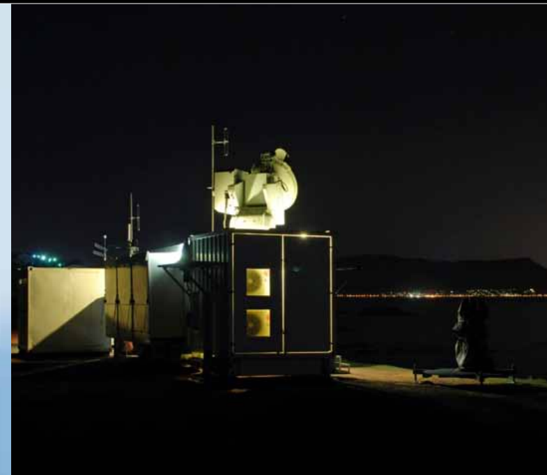
The MecORT R&D laboratory deployed outside Simons Town in False Bay during May 2008. Radar data was recorded in support of R&D on small boat detection in sea clutter and radar target recognition using high range resolution and inverse synthetic radar (ISAR) processing.
