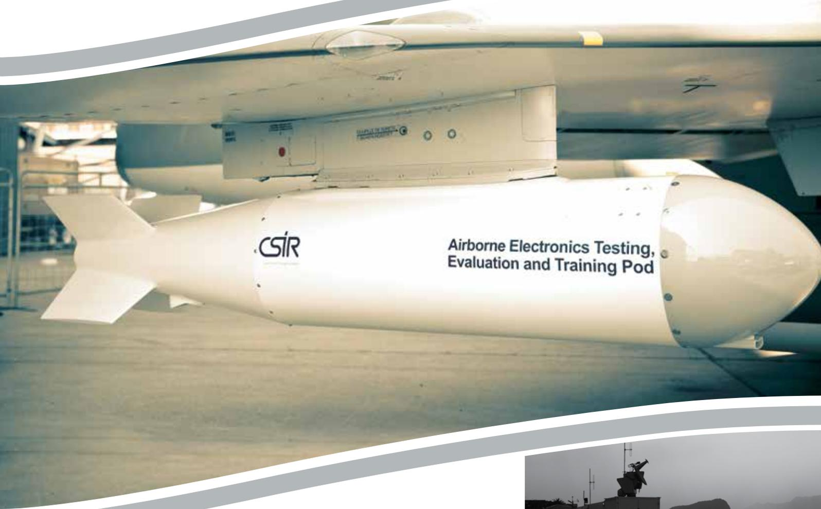
Inundu is a multi-purpose electronics pod for airborne Electronic Warfare (EW) and Radar test evaluation (T&E) and training applications. The modular payload can be re-configured for various research, development, test, evaluation and training scenarios.
