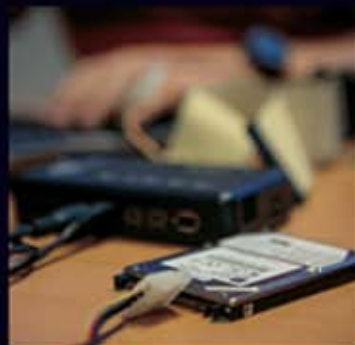
An unsecured printer hard drive being scanned for sensitive information.
